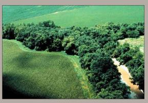
I-14: Hedgerows or trees are used to help stabilize soils and trap sediment movement.
