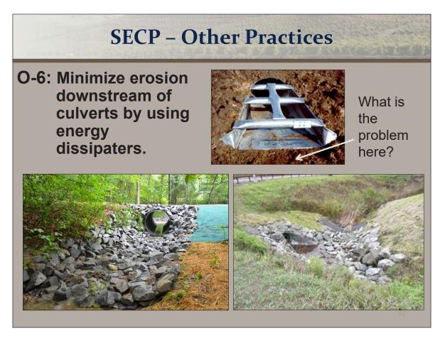
O-6: Minimize erosion downstream of culverts by using energy dissipaters.
