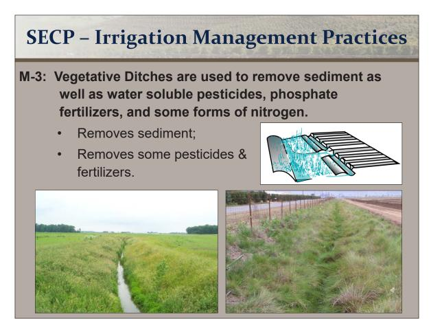
M-3: Vegetated ditches are used to remove sediment as well as water soluble pesticides, phosphate fertilizers, and some forms of nitrogen.
