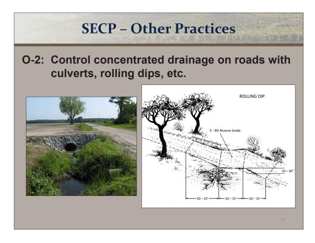
*O-2:* Control concentrated drainage on roads with culverts, rolling dips, etc.
