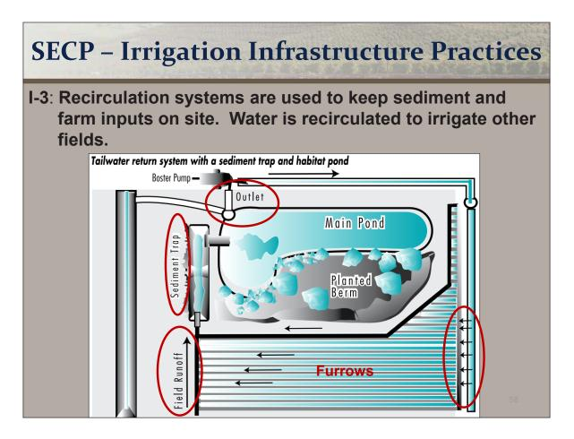
I-3: Recirculation systems are used to keep sediment and farm inputs on site. Water is recirculated to irrigate other fields.
