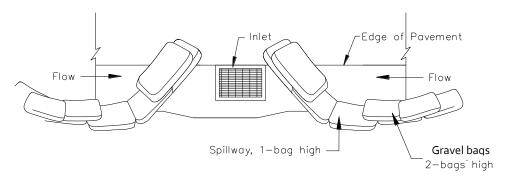
TYPICAL PROTECTION FOR INLET ON SUMP
