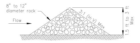
TYPICAL ROCK CHECK DAM SECTION
