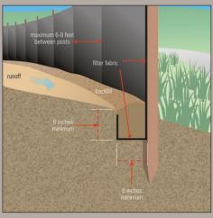
Installation of silt fences is a common practice used to mitigate sediment discharge of sheet flow.
